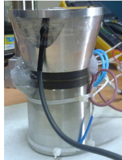
Fig. 5. Manufactured transducer according to simulation.
