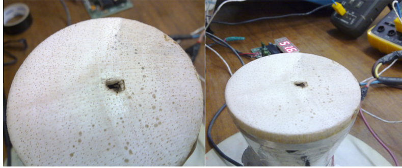
Fig. 10. Burned wooden matching layer at 300 W of power.
